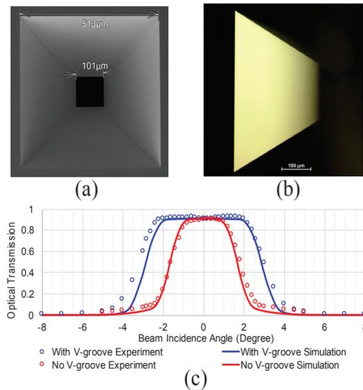
**FIGURE 3.** (a) Top view and (b) side view of an etched Si V-shaped cavity; (c) experimental vs. simulation results indicate  $>100\%$  improvement on acceptance angle and  $CAP$  by incorporating the low-profile Si cavity into a traditional optical concentrator system.
