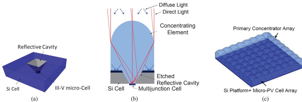
**FIGURE 2.** (a) A novel multi-functional Si cell platform that integrates an array of concentrated multijunction micro-cells; (b)&(c) a baseline structure consists of a molded lens array layer, a multi-functional Si cell, and an integrated array of high concentration multijunction micro-cells.
