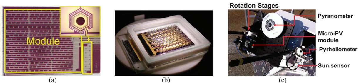
**FIGURE 1.** Prototype micro-scale CPV modules developed in the Microsystem-enabled Photovoltaic program: (a) prototypical module integrating molded micro-concentrating optics and micro-cell arrays; (b) fabricated micro-cell array and interconnects; (c) on-sun characterization setup.
