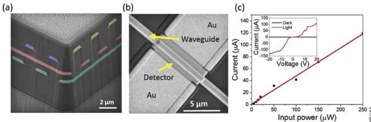
Figure 1. (a) Tilted focused-ion-beam SEM view of a multilayer woodpile photonic crystal (before delamination from the silicon handler substrate). Colors indicate various layers.<sup>2</sup> (b) SEM image of a chalcogenide glass waveguide integrated photodetector. (c) Measured photocurrent of the photodetector as a function of waveguided optical power at 1550-nm wavelength. Inset shows *I*-*V* characteristics of the detector in dark and at 250-μW input optical power.
