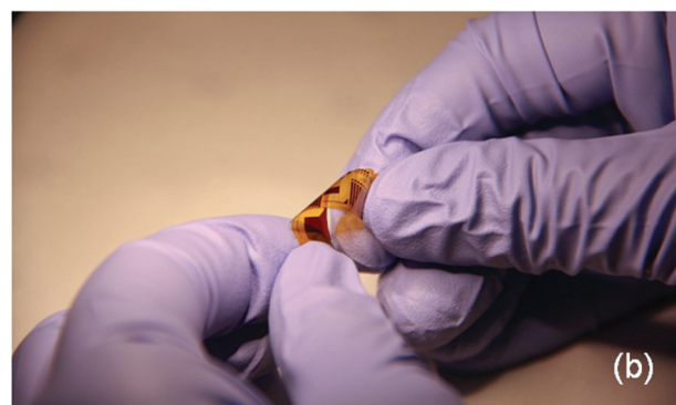
Figure 3. (a) Fabrication process for ChG flexible photonic devices. (b) Example of a flexible photonic chip. 11
